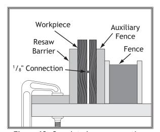
Figure 62. Completed resaw operation.
